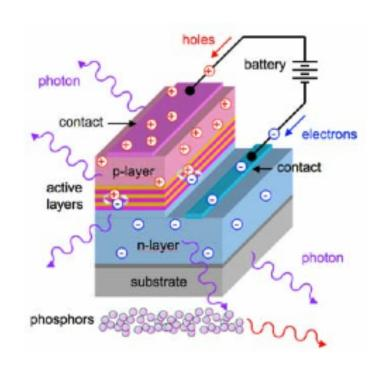
Current white LEDs are InGaN blue with YAG based phosphors
