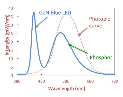
High colour temperatures; CCT ~4000K Poor colour rendering; CRI ~ 80
