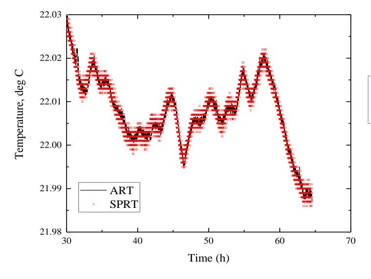
Resolution of < 1 mK temperatures at room temperatures
