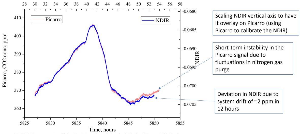
ART NDIR Picarro comparison with Sapphire windows 60 cm tube heated to 40 deg C and N2 purge 09\_01\_19.opj
