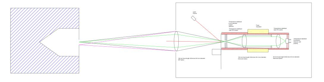
Development of the Ambient Radiation Thermometer 8 um to 14 um filter ZnSe lenses Pyroelectric detector
