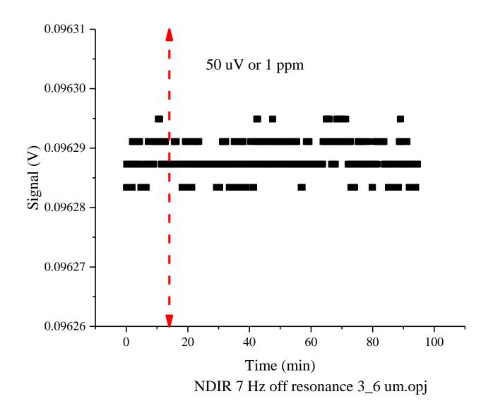
Off-resonance signal stability is 0.2 ppm of CO2 for hours
