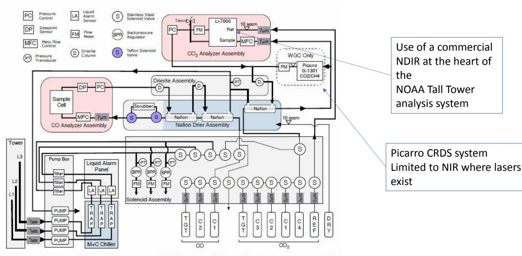
Fig. 1. Schematic diagram of the NOAA ESRL Tall Tower CO<sub>2</sub>/CO analysis system. The Picarro G-1301 analyzer is only included at the WGC tall tower site (Walnut Grove, CA). Line thickness indicates tubing diameters of 0.125, 0.25, and 0.375 in. (0.3175, 0.635, 0.9525 cm). Pink and blue shading indicate heated and cooled enclosures. Photos are provided in the supplementary material.
