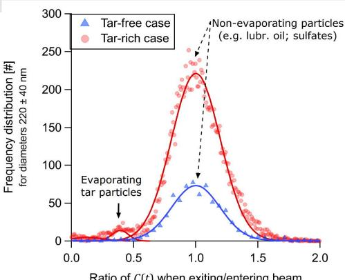
Ratio of C(t) when exiting/entering beam R(20%, -20%) [-]
