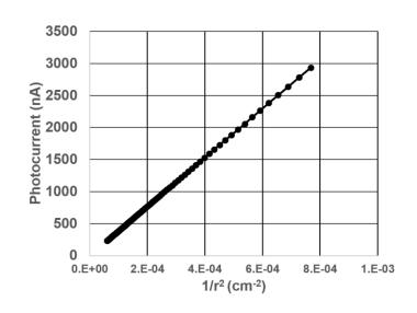
We choose the COBs with symmetric angular profile and linear distance dependence
