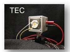
Mounts with cooling modules for the COBs
