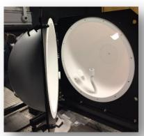
50cm sphere for  $4\pi$  and  $2\pi$  LED total flux measurement
