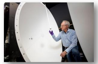
1.6m sphere for  $4\pi$  and  $2\pi$  LED total flux measurement
