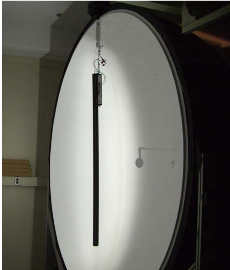
Measuring a refrigerator LED luminaire
