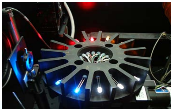
Variable temperature chamber ( \sim 10^{\circ}\text{C} to 35^{\circ}\text{C} )
